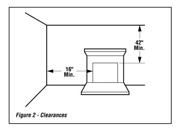
**Step 2. Ceiling Clearance:** The ceiling must be at least 42" from the top of the appliance opening (*Figure 2*).
